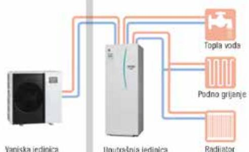
SISTEM SPLIT TOPLITNE PUMPE SA UNUTRAŠNjom JEDINICOM HIDROBOX I ODOVOJENIM SPREMNIKOM PTV
